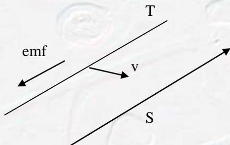
Figure 1-2: Target motion induction
