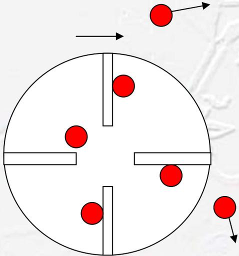
**Figure 4-2: Coriolis wheel**
