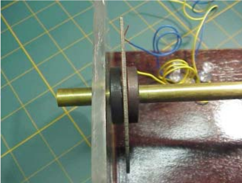
Figure 2-2: Close-up shows that disk is sandwiched by two disk magnets (note old brush configuration )
