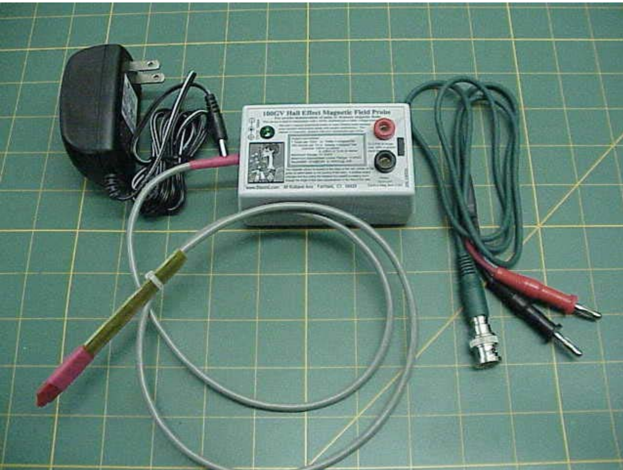
Figure 1-1 The 100GV kit (The probe shows a white cable tie use to protect the probe during shipment)
