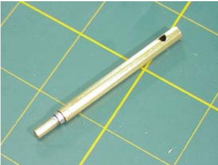
Figure 3-15: The completed drive shaft
