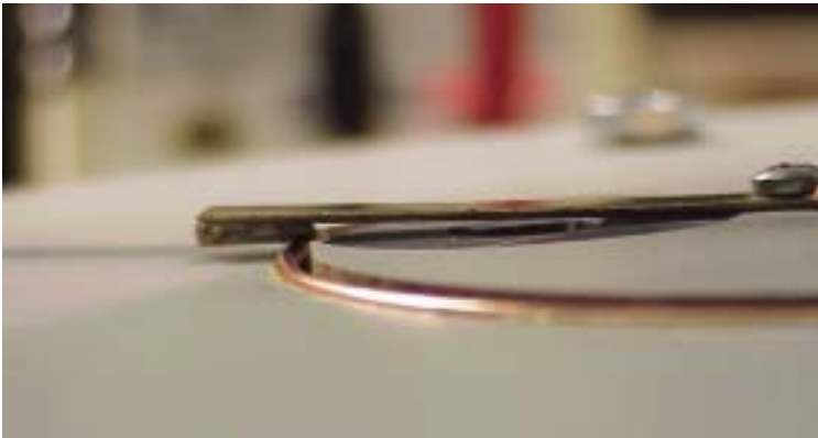
Figure 3-30: Stator Ring tension before adjustment
