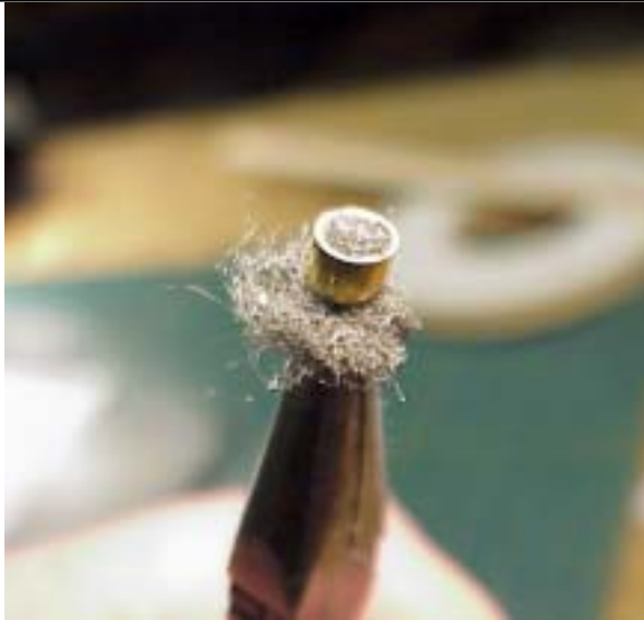
Figure 3-5: cleaning the inside of tubes (usually just the ends)
