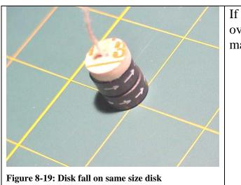
If the test disk were slowly lowered over a disk of the same diameter, it maximizes edge to edge alignment.
