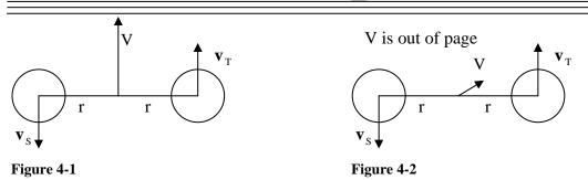
For Figure 4-1 and Figure 4-2, the equation (of step 4) resolves to  $V_t^2 = C^2 - V^2$  without intervention. For readers who wish more background with the BMP in motion, the system of Figure 4-2 is solved in the paper titled "New Gravity"—(ng.pdf).
