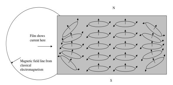
Figure 8-10: Edge current of single magnet.
