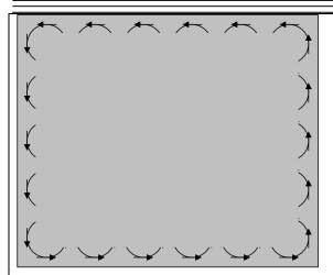
Figure 8-2: Effective current (Edge Current)
