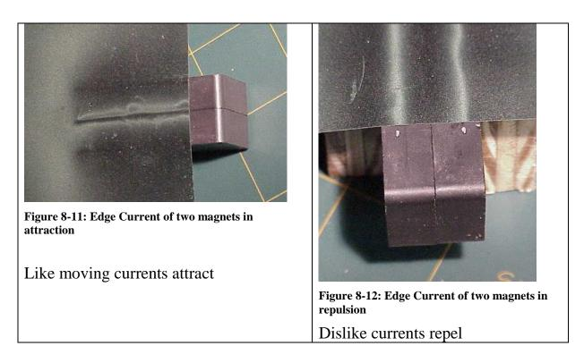
In Figure 8-11, the edge currents of the two magnets are drawn toward each other; likewise, if the magnets are in repulsion as shown in Figure 8-12, the edge currents are pushed away from each other.
