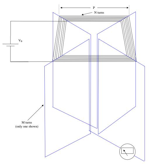
Figure 11-1: Corner Effect Transformer
