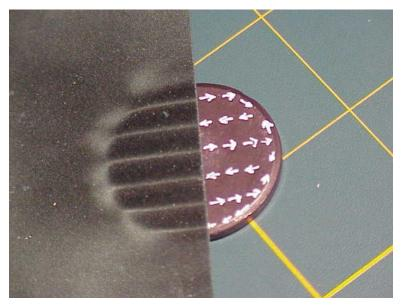
Figure 8-15: Disc magnet with non-standard domains
