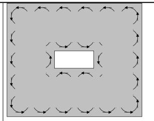
Figure 8-3 Effective current of magnet with hole.
