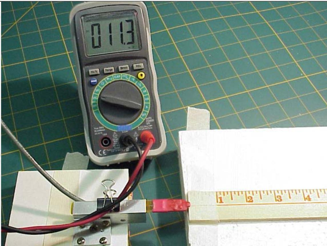
Figure 1-2: Setup to measure flat magnets
