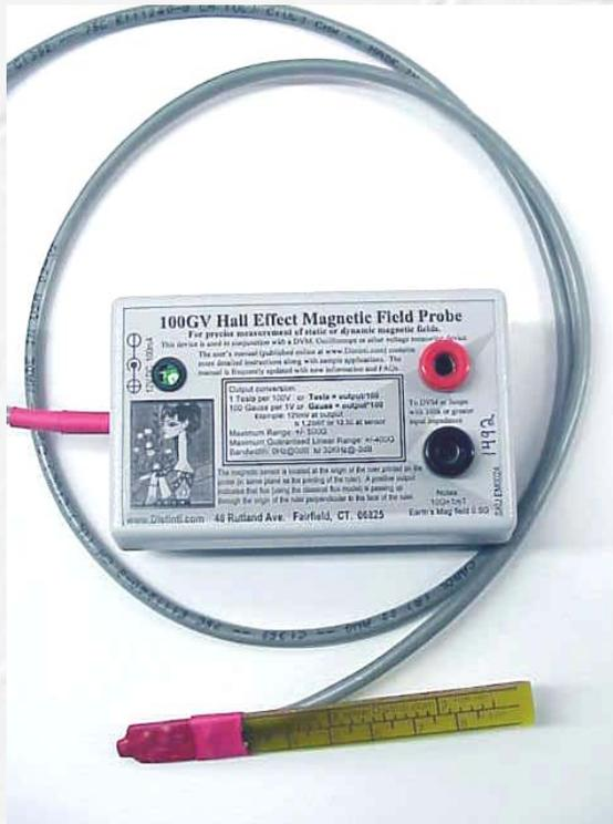
Figure 1-1: The 100GV Hall Effect probe
